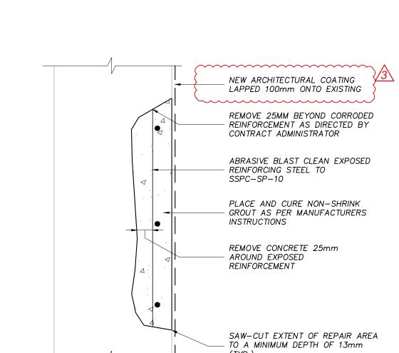
TRENCH DRAIN REPAIR SECTION
