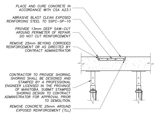
3 TYPICAL TOP SURFACE REPAIR DETAIL S2 / SCALE: 1:16
