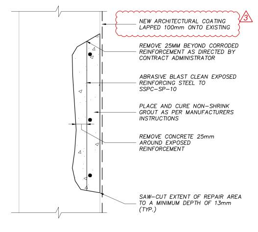
5 TYPICAL CONCRETE WALL REPAIR DETAIL
