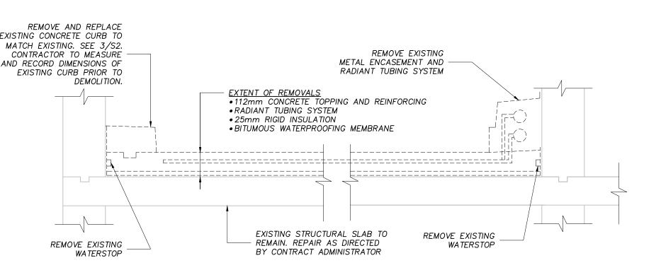
TYP. RAMP DEMOLITION/REMOVALS SECTION SCALE: 1:16
